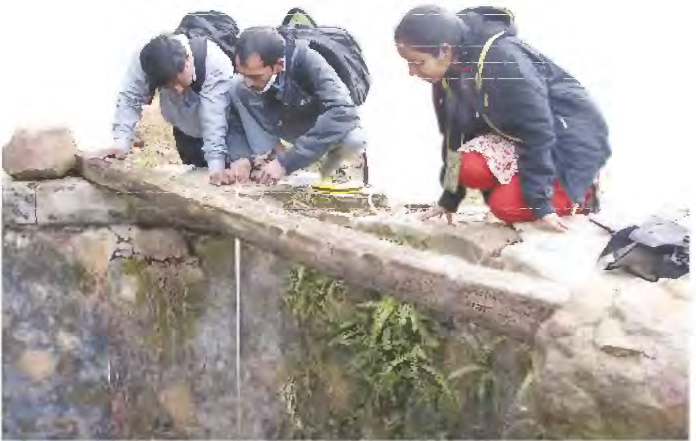
Measuring depth of water of well for plotting water levels in Dumka block, Jharkhand, Name of partner: PRADAN
